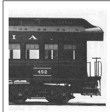
A *Pennsylvania* Railroad coach, 1879, showing "porch" style vestibule, with steps, guardrail, hand brake, and overhang, from John H. White, Jr., Vol. 1, p.93
