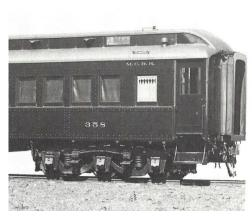
A *New York Central* coach, 1921, showing vertical end-frame flexible connector for enclosed vestibule, from John H. White, Jr., Vol. 1, p.156
